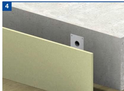
Position compressible joint filler of the appropriate width, for applications where movement is expected between the two sections of concrete.
