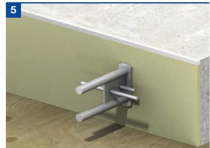
Push the dowel component through the joint filler (if applicable) until it is fully located in the sleeve component. It may be necessary to tap the dowel component to overcome the dimple which pinch holds the dowel in the sleeve and prevents dislocation when the concrete is vibrated.
