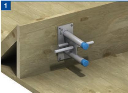
Nail the sleeve component to the shutter ensuring that the sleeve is correctly orientated for the direction of the load. Check that the minimum spacing and edge distances are not exceeded. The label prevents debris from entering into the sleeve aperture and should not be removed at this stage.
